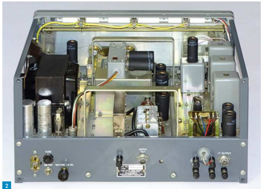
Fig. 1: The EA12 has a wide range of features for AM, SSB and CW reception. Fig. 2: The heart of the EA12 is a diecast coil box carrying the RF stages, flanked by two subchassis and secured to a sturdy front panel. Fig. 3: The date of manufacture can be deduced from the EA12 Serial No. Fig. 4: The ratio arm (arrowed) produces a near-linear frequency tuning scale.
