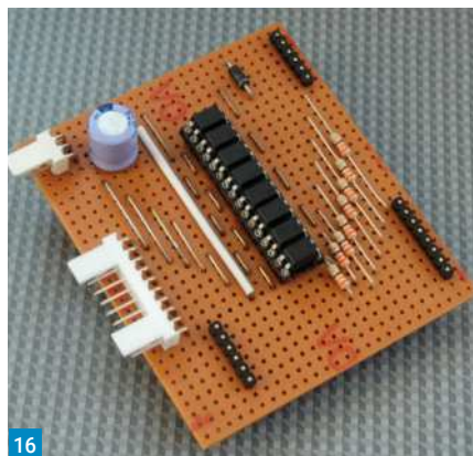
Fig. 16: Slave top shield. Fig. 17: Circuit diagram of the slave unit. Fig. 18: Relay board. Fig. 19: Position of components as seen from above, also details of multi-way cable connecting the relay driver to the relay board. Fig. 20: Master unit rear. Fig. 21: Slave unit.
